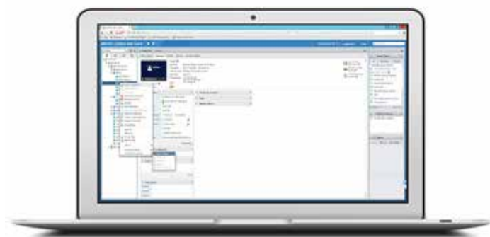
Fig. 2 » Velostrata vCenter Plug-In. Right-click VMs to “run in cloud” or “run on-premises.”
